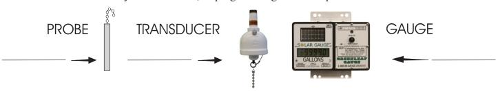
1. The gauge has been pre-programmed and put into a <u>"SLEEP MODE"</u> for storage and shipping to preserve power. Sleep mode will constantly display the Program Version, i.e. 80-E. To wake up the gauge: Use the pocket magnet to touch the PLANET symbol on the front of the gauge. Hold only until the gauge display changes to the Firmware version, i.e. 11 - 00 or similar. Pull away the magnet and it will go to normal operating mode.
