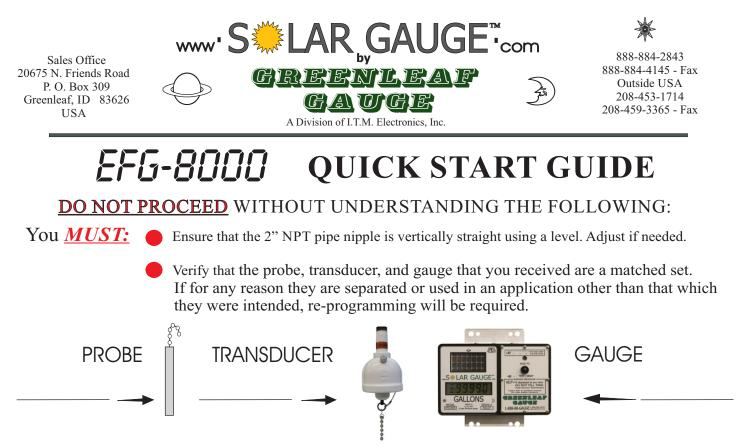
The gauge has been pre-programmed and put into a <u>"SLEEP MODE</u>" for storage and shipping to preserve power. Sleep mode will constantly display the Program Version, i.e. 80-E. To wake up the gauge: Use the pocket magnet to touch the PLANET symbol → on the front of the gauge. Hold only until the gauge display changes to the Firmware version, i.e. 11 - 00 or similar. Pull away the magnet and it will go to normal operating mode.
