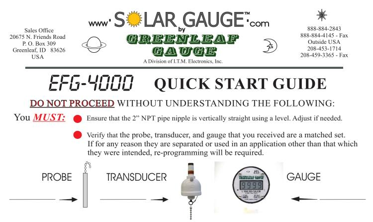
The gauge has been pre-programmed and put into a <u>"SLEEP MODE</u>" for storage and shipping to preserve power. Sleep mode will constantly display the Program Version, i.e. 40-4. To wake up the gauge: Use the pocket magnet to touch the PLANET symbol
